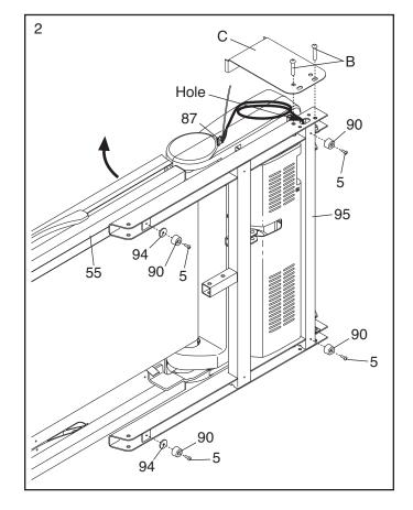
3. **See the inset drawing.** Cut the plastic tie near the Upright Wire (87).
